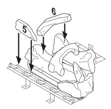
Figure 49 - Installing Logs No. 5 and No. 6
